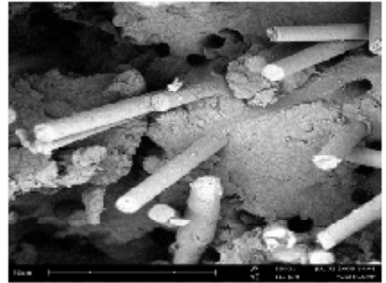
Figure 1: Tensile Properties of Composites vs. Fiber Weight Fraction. Adjacent, Scanning Electron Micrograph of the Fiber-Matrix Interface
