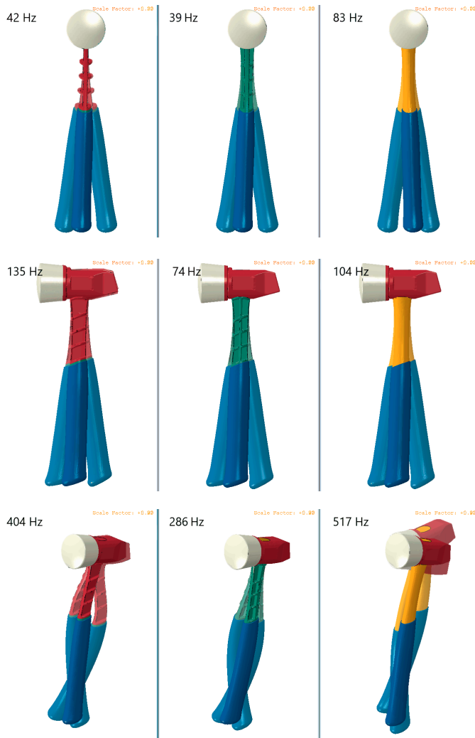
Figure 20: Eigenmodes and eigenfrequencies for hammer shafts (left to right: steel, polymer, wood)
