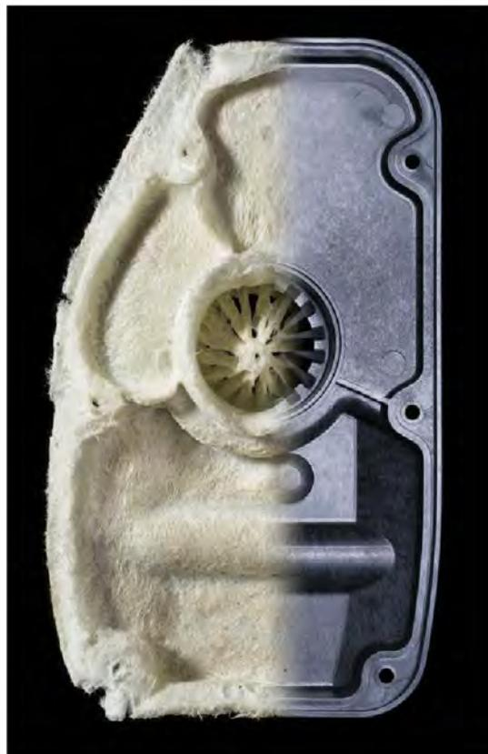
Burning away the plastic substrate of an injection molded part using pyrolysis reveals the internal fiber skeleton which is providing reinforcement. This method can be used to check for even fiber distribution and fiber alignment at key stress points. Source: PlastiComp
