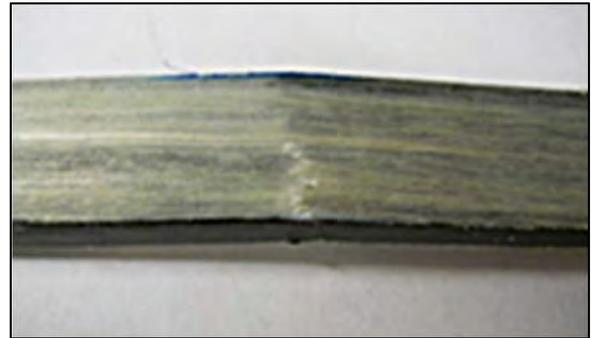
Figure 4: Failure of injection-molded test-bar underlying material; tape holds fractured halves together suppressing catastrophic failure.
