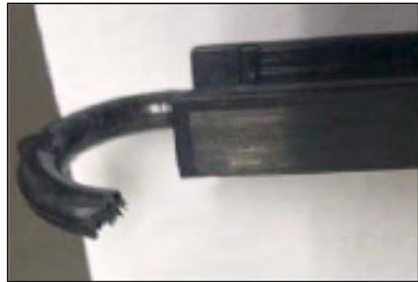
Figure 2: (A) Injection molded I-beam in 3-point bend testing and (B) tape insert in as-molded I-beam.
