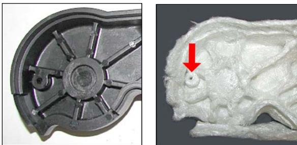
*Figure 8. As molded and fibrous skeleton showing how fine features such as a pin boss are maintained due to the skeletal network of the long fibers (long glass fiber in PES resin)*
